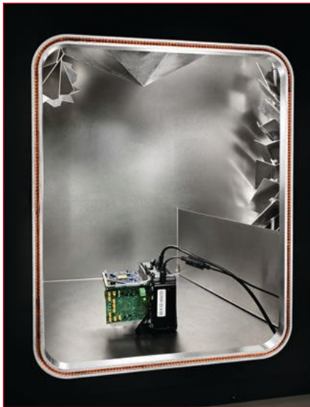
▲ Fig. 6 Pharrowtech 60 GHz PTK1060 and mode stirrers. 5
